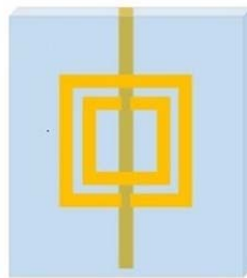
Fig. 10: Schematic of a single resonating structure (usually called a unit cell) in a metamaterial. It is composed of a dielectric substrate in between (as shown in blue) and copper wire (as shown in golden) on one side of the substrate and on the other side copper rings (as shown in yellow). Metamaterials are composed of period arrangement of such structures in different directions. (Image courtesy: Google Images)
