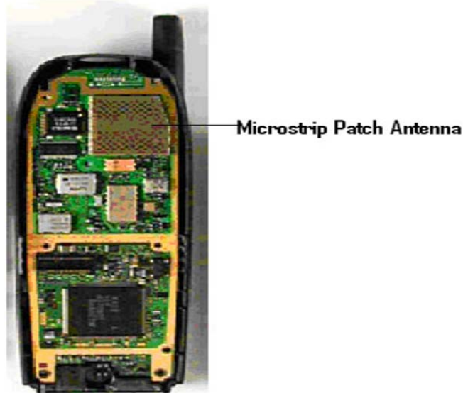
Fig. 4: Patch antenna in mobile handset.
